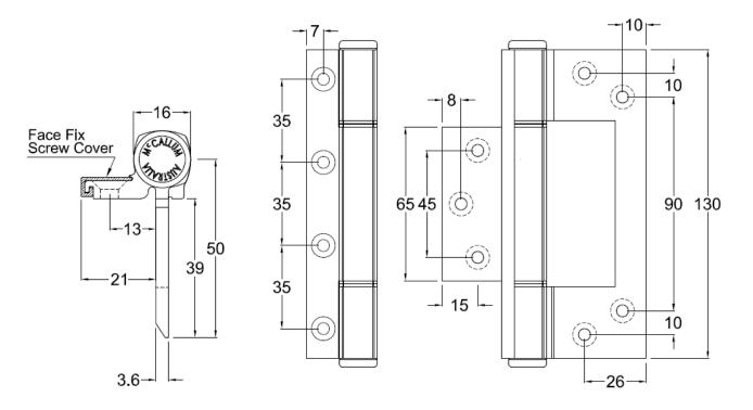
The A13040 Aluminium Frame-Fold Interleaf hinge has been designed to take the Wrap-around face fixing to the next level by introducing a cover plate for the concealing of the face fixing screws, improving the aesthetics while maintaining the strength and durability.
