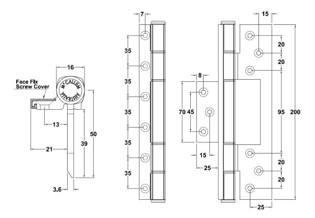
The A20040 Aluminium Interfold hinge has primarily been designed for larger & heavier doors A unique five-knuckle design for enhanced strength and durability, while improving the aesthetics via a cover plate concealing the framefold face fixing screws.
