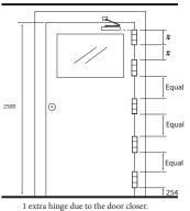
Number of Hinges Required per Door Size 820 (W) 2100 mm (H) 3 2300 mm (H) 4 2500 mm (H)
