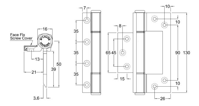
The A13040 Aluminium Frame-Fold Interleaf hinge has been designed to take the Wraparound face fixing to the next level by introducing a cover plate for the concealing of the face fixing screws, improving the aesthetics while maintaining the strength and durability.
